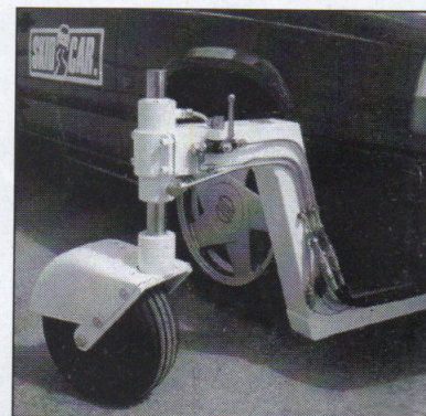
Hydraulic ram with pivot wheel. With the lever you select split-friction and over/under steering.
