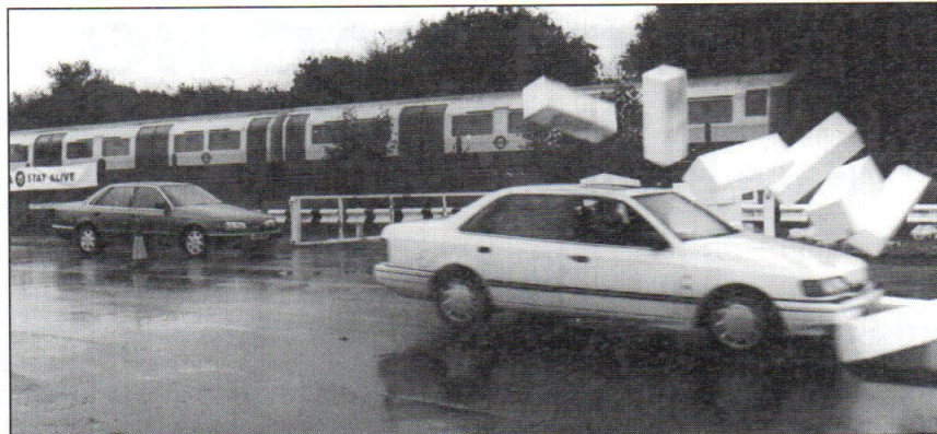
Police drivers test bald tyres at the Hendon Police Driving Centre. The car with the illegal tyres crashed through the polystyrene wall.
